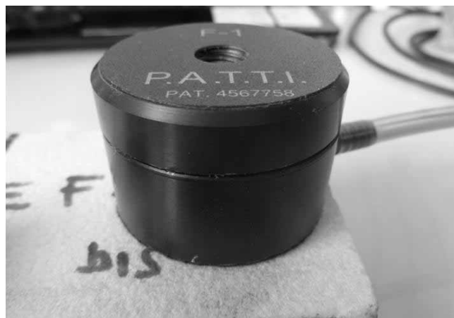
Fig. 3 Pneumatic adhesion tensile testing instrument (PATTI)
