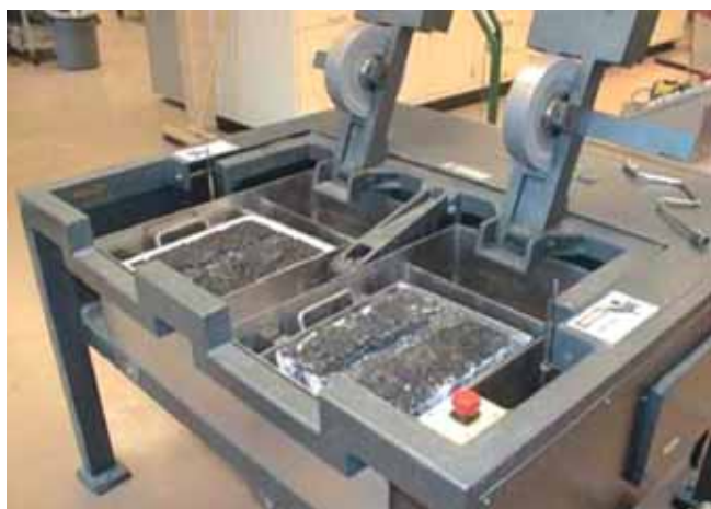
Fig. 2 Dispositivo HWTD (Hamburg Wheel Tracking Device)
