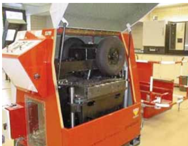
Fig. 4 Dispositivo FRT (French Rutting Tester)
