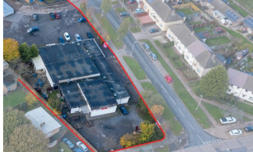
760 m 2 cold flat roof (33 tonnes)
