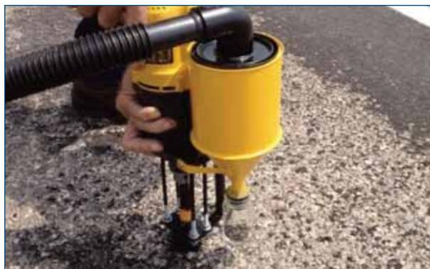
**Fig. 9** Micro-sampling, non-destructive coring technique
